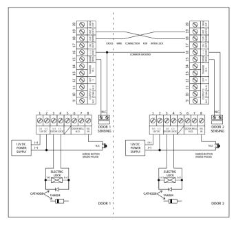
An inter-lock system needs two door controllers. This application example uses two keypads with simple cross wire connection on their "Output 1 INHIBIT" and "Inter-lock Control Output" terminals. It is necessary to link up the "(-) GND" terminals of the two keypads as common ground to achieve the inter-lock logical functions.
