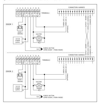
An inter-lock system needs two door controllers. This application example uses two DK-9823 with simple cross wire connection on their "Output 1 INHIBIT" and "Inter-lock Control Output" terminals. It is necessary to link up the "(-) GND" terminals of the two keypads as common ground to achieve the inter-lock logical functions. The connection of the Green LED is optional. It lights up for lock energized.
