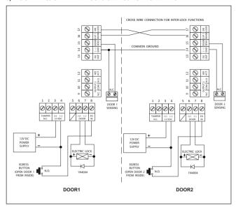
An inter-lock system needs two door controllers. This application example uses two keypads with simple cross wire connection on their "Output 1 INHIBIT" and "Inter-lock Control Output" terminals. It is necessary to link up the "(-) GND" terminals of the two keypads as common ground to achieve the inter-lock logical functions.
